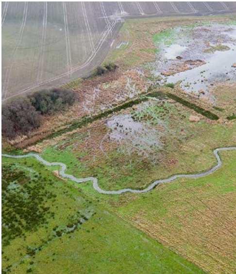
The natural hydrology has been recreated in the river valley along Kapelbæk near Langballe and Beder. Now, the former ditched stream is once again meandering through the terrain.
